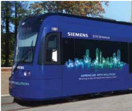
The interior of this S70 streetcar has been designed to maximize passenger space, incorporating a predominately knee-to-back seating arrangement. Each S70 Streetcar is equipped with eight (8) wide opening sliding plug doors all located in the low floor area, with four (4) to each side of the vehicle. The door spacing has been optimized to allow for greater passenger flow entering and exiting the vehicle, which ultimately decreases the station dwell times.
